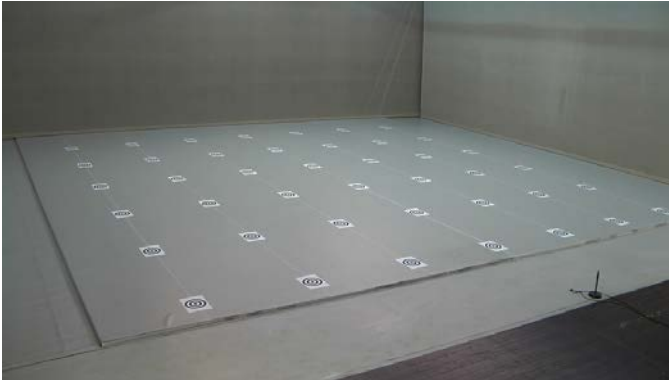
Fig. 3: Use of spherical markers for estimation of the camera poses in relation to each other.
