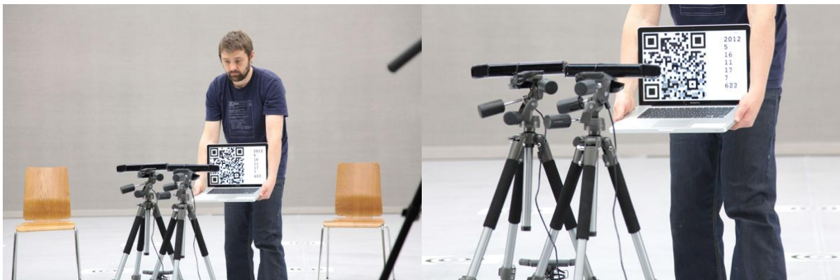
Figure 4: QR code used for camera synchronization.
